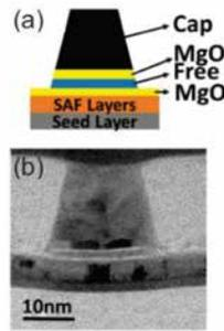
Figure 2: Illustration of proposed NV-BNN architecture. Schematic and TEM image of p-magnetic tunnel junction device exploited [2].
