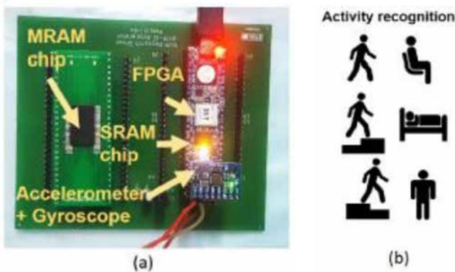
Figure 3: (a) Inference Accelerator test-bench for memory evaluation for NVIA concept. (b) Classes of HAR dataset. [3].
