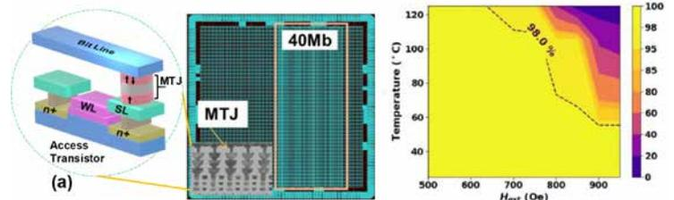
Figure 4: (a) 22nm FD-SOI based 40Mb MRAM macro (Inset: TEM Image of MTJ arrays) and MRAM device schematic. (b) Contour plot showing impact of temperature and external B field on inference accuracy of the binarized CNN [4].
