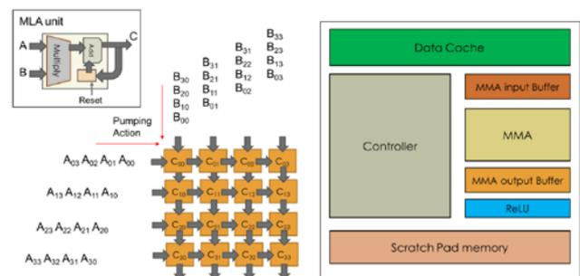
Figure 1: Data flow and blocks of proposed systolic accelerator. Memory blocks including NVM and SRAM were investigated [1].
